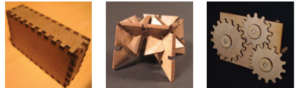
Figure 1. Physical output of FlatCAD: parametric boxes, polygon construction kit, mechanical gears.
