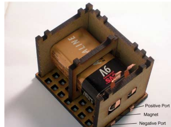
Figure 3: The CHI BOX connection ports on the right side are made by copper foil tape.
