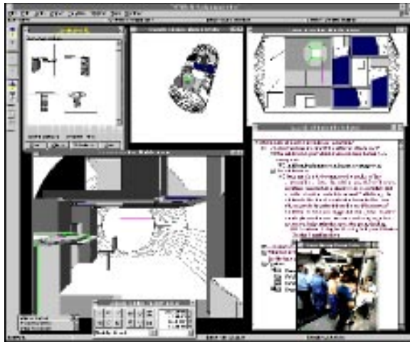
Figure 3. The PHIDIAS HyperCAD system structures a database of design artifacts and argumentation.
