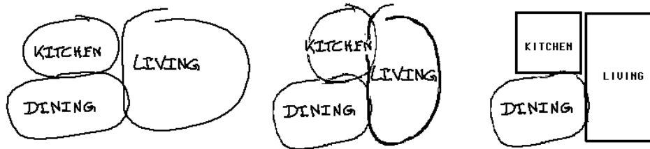
Figure 6. Stretch-A-Sketch maintains relations in the diagram. (a) diagram as first drawn; (b) after resizing a room; (c) partially rectified drawing.
