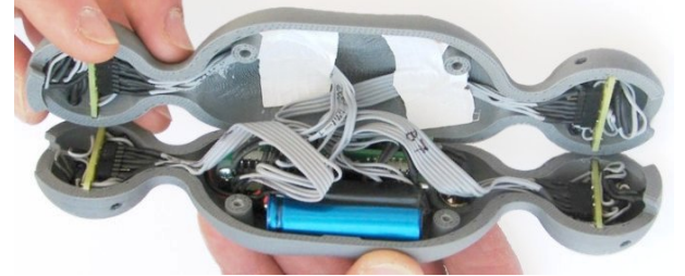
Figure 7: Strut shell open to show electronics inside.
