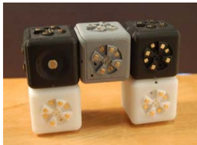
Figure 4. A mobile robot that steers away from light sources.
