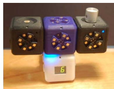
Figure 3. A little robot that indicates a number based on the values of two connected sensor blocks.
