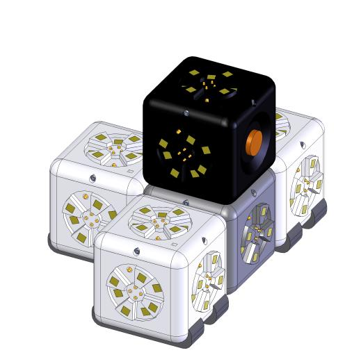
This robot drives forward at a speed corresponding to the amount of light in front of it.
