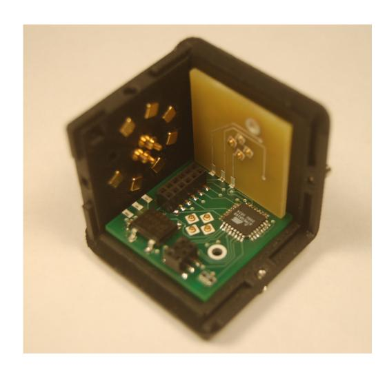
Each block contains an AVR microcontroller, LEDs, power circuitry, and six printed circuit boards.
