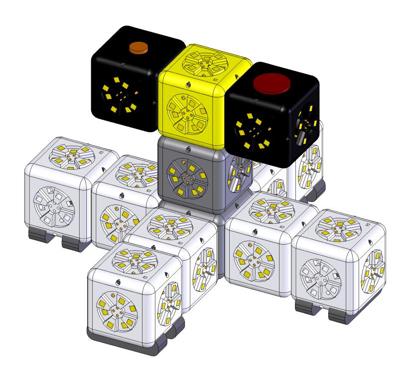
This robot spins in place at a rate corresponding to the total ambient light and sound in the environment.
