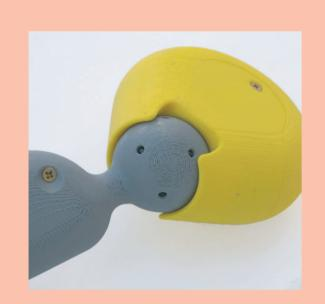
LEDs embedded in each ball send serial data to photosensors in each socket.
