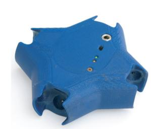
The Posey construction kit is composed of hubs and struts with poseable optocoupled ball and socket connectors.
