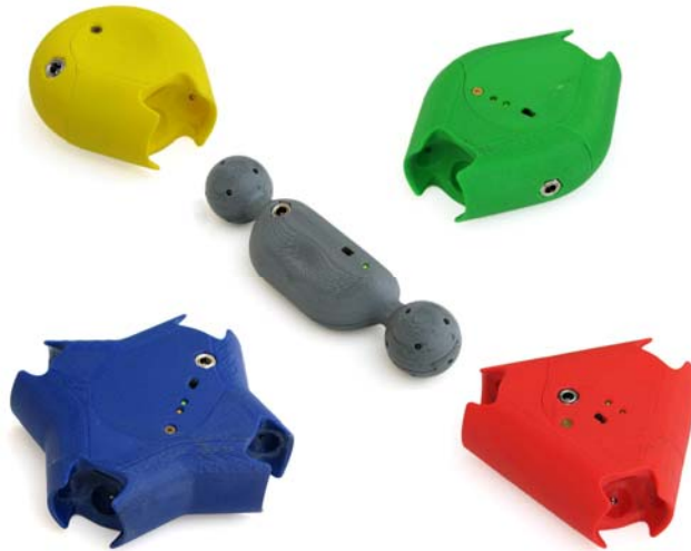
Figure 4. Posey consists of hubs and struts that connect in ball-and-socket joints that are instrumented with an optocoupler.
