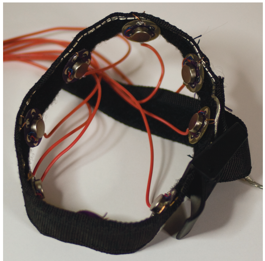
Eight LilyPad tactors arranged in a compass formation, driven by an Arduino Mega. The next iteration will use EAI tactors or similar commercial device.
