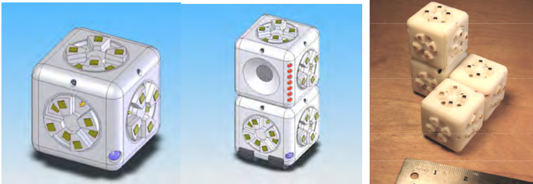
Figure 11. Two more early prototypes of construction block interfaces. Top: narrative blocks through which elements of simple animations can be chosen by the orientation of a block interface. Bottom: design for "Roblocks", a set of building blocks that contain sensors, actuators, and logic, and that can be connected into complex robotic constructions. At bottom right, the first physical prototype of Roblocks.
