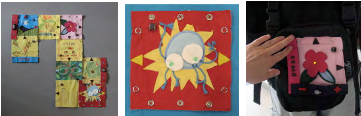
Figure 2. Quilt Snaps: a medium for constructing programmed behavior from decorated fabric patches. At left, a quilt construction; at center, a close-up of a decorated patch; at right, a patch snapped onto a backpack.
