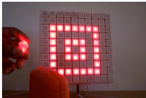
Figure 12: SmartTiles. Upper row: a ten-by-ten array of the tiles running a Game of Life cellular automaton. Center and bottom rows: a wireless "color transmitter" built into an ambient pendant is brought close to one of the SmartTiles; this new version of the tile has an infrared receiver that enables it to "read" its color state from an external source. In the bottom row, the entire array is now propagating "waves" of the color as a result of the cellular automaton rules contained in the tiles.
