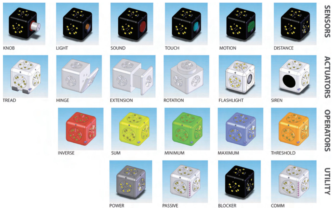
The catalog of roBlock types: sensors, actuators, operators and utility blocks.
