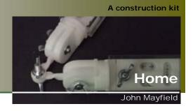
T-C Members are individual truss members which, when loaded, indicate mechanically whether they are in tension or compression. They can be assembled into complex 2D and 3D trusses. They are intended to be used as a learning tool.
