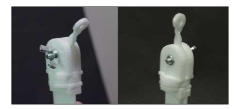
The upper hinge is simply a bit of threaded rod through four layers of plexi. By adding a wing nut, to one end, and embedding a bolt in the outermost layer of plexiglass on the other, this hinge can be tightened to restrict movement. The answer to that range of motion problem.
