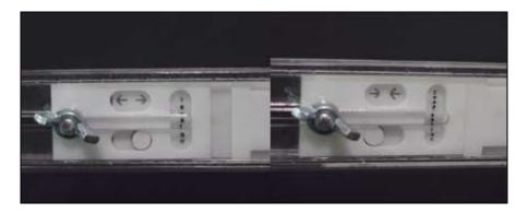
The indicator change was an attempt to make that part of the member more rugged. One of the intermediate steps between the early version and this one was the miniaturization of the early indicator switch. I found that the change in size made certain parts of the assembly too fragile to hold up under stress.
