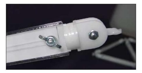
Perhaps most seriously, and most noticeably, the eyelets of the connectors tend to break off. I am, at this point, unsure if this is simply because of how thin these pieces are, or if it might have something to do with their being melted and twisted. I don't know whether this heating process might have weakened the plastic.
