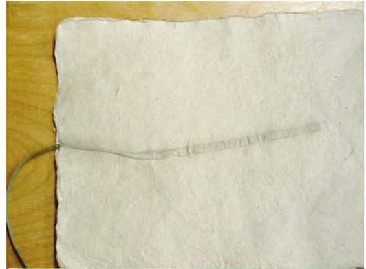
Figure 3 Test sheet of paper with the form of the bend sensor digitally highlighted
