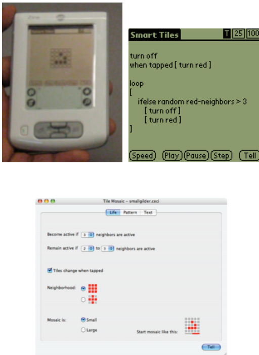
Figure 6. Three types of SmartTile programming: setting initial configurations of "live" and "dead" cells (upper left); textual programming (upper right); and menu-driven interface (bottom).
