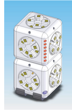
Figure 1. A light sensor atop a twisty block turns toward light.
