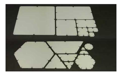
Floor and ceiling panels came in two main types: 90-degree and 60-degree. The 90-degree panels are either squares or 2:1 rectangles with dimensions of 5, 10, 20 and 40 feet. The 60-degree panels are made up of hexagons, trapezoids, and triangles, also having side dimensions of 5, 10, 20 and 40 feet. Each side with a length of 10 feet or more is further subdivided by a connector at it's center. This allows for more flexible connections between pieces of different dimensions.
