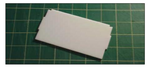
The floor, ceiling, and wall panels were made from 1/8" thick plexiglass. The panels were laser cut from 18" x 36" sheets to create the exact shapes needed. The cutting took roughly 30 hours.
