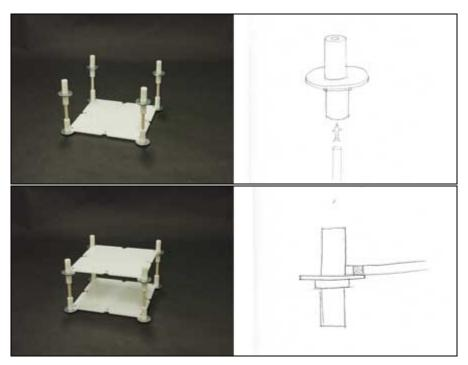
The dowels are then topped with double sided connectors. Be sure to orient the double sided connectors such that the washer is above the plastic ring.
