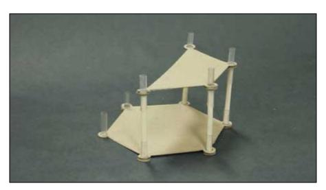
The connections were all non-permanent. A floor panel would slip over a set of base connectors, which could then each hold columns. The columns could then receive two-sided connectors, on which could go another floor and ceiling panel. The connection was such that multiple panels could meet at each connector, and overlap as they connected to it.
