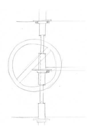
A similar problem arises when attempting to position a 20' tall wall panel next to two 10' wall panels. The connector required to hold the corner of the lower 10' panel interferes with the 20' panel.
