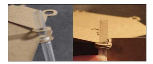
I found that problems arose when attempting to connect the wall panels to the ceiling panels and connectors. When designing the kit, I had assumed the thickness of 1-dot chipboard to be negligible, but I quickly found that a few overlapping ceiling connections, combined with the thickness of the connector could make attaching wall panels difficult, or even impossible.
