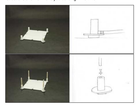
Begin by attaching base connectors to a floor panel. The base connectors should be on the ground with their cylindrical ends pointed upward. The floor panel then attaches magnetically to the connectors by simply resting each corner (or side connection) on top of the metal washer.
