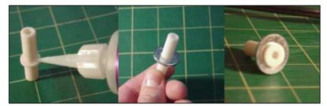
Each washer was then glued into place, and 1/3 of the connectors were cut in half to serve as base connectors. Finally my kit was complete.
