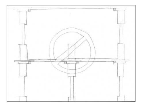
The first problem is that it is not possible to position a longer panel above two smaller panels. The middle connector required to hang the smaller panels will stick up into the space of the larger panel.
