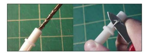
As I said, though, the door guides were close, but not perfect. The three main problems with them being that the diameter of the inner hole would not work well with any standard dowel size, that there was an inner plug but it was not centered, and that there were ridges along the outside of one end.
