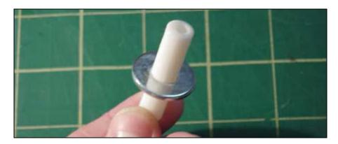
The connectors were the most challenging piece to create, due to their unusual shape and requirements. They are basically just hollow cylinders, but with a metal washer around the outside, supported by a small plastic ring. Additionally, the hole of the cylinder had to be a very specific diameter to accommodate the dowels that would serve as columns, and had to have a stopper at mid-height to prevent the columns from slipping through.
