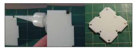
1/8" Nickel-plated neodymium magnets, which would serve as the basis of all connections were then glued in place using cyanoacrylates (crazy glue). Keeping the magnets all properly aligned was something of a challenge, but I was able to determine the direction of each magnet's poles by setting them each on a larger magnet prior to gluing them in place.
