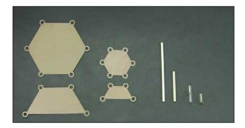
The system in which I was attempting to design allowed only for hexagonal and trapezoidal floor and ceiling panels. I found that a remarkable variety of building forms could be derived from these simple shapes. One of the main virtues of the hexagon is that when bisected across two intersections, the resulting side is twice the length of the original sides. That is to say, that the long sides of the trapezoids are exactly twice the length of the three other sides.
