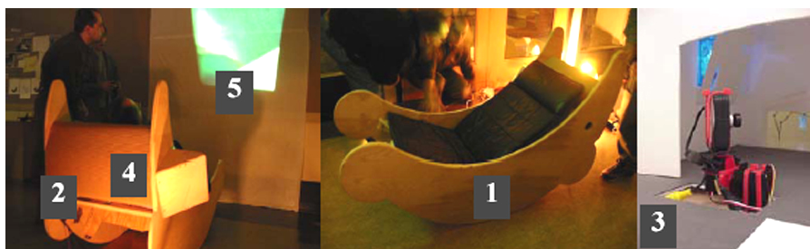
Figure 8. Window Seat components: (1) physical chair; (2) handyboard microcontroller; (3) remote camera; (4) projector; (5) wall as display device
