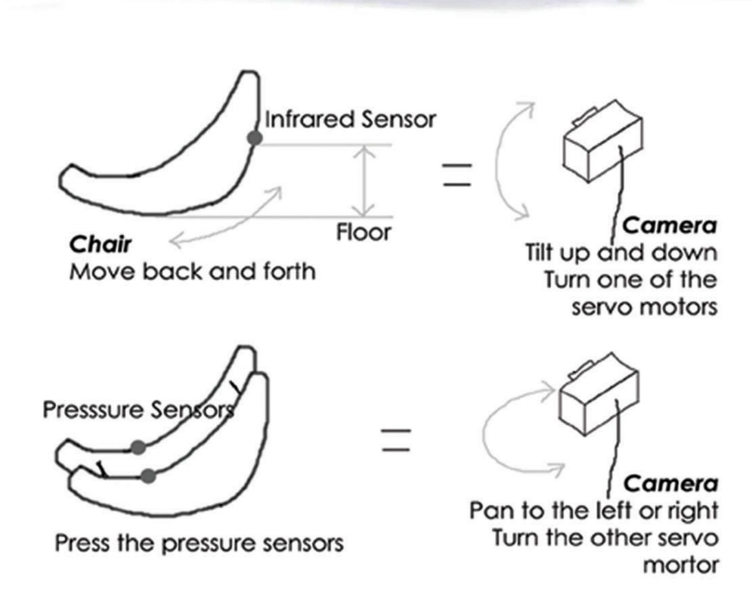
Controlled by the sensor values, two servo motors mounted at a right angle drive the camera in two axes (tilt and pan).
