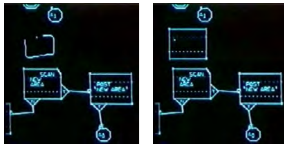
Fig. 1.2 On left, a GRAIL user draws a model element in place. At right, the rectified element is displayed as a box.
