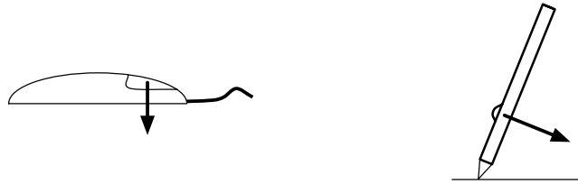
(a) Pressing a mouse button exerts force perpendicular to the operating plane.
