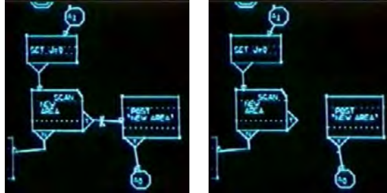
Fig. 1.3 GRAIL’s sketch interpretation is context sensitive. At left the user crosses out the connector, which is interpreted as a delete command, shown at right.
