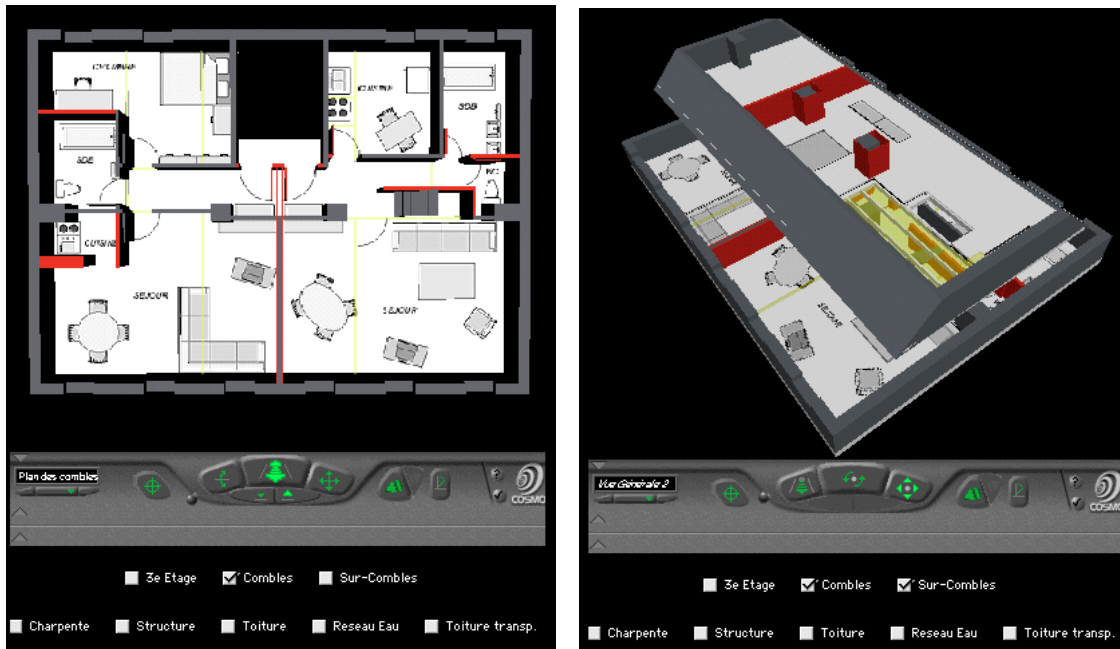
Figure 7: Design Phase I (Hybrid representation). The 3-D model of the existing building embedded with several layers (checkboxes at the bottom of the browser) for participants to explore different design issues. Left: floor plan with furniture layout. Right: the relationships between two floors.
