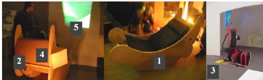
Figure 2. Chairware Components; (1) Physical chair; (2) Handyboard; (3) Remote Camera; (4) Projector; (5) Wall as Display Device
