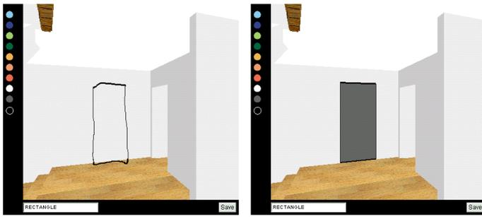
Figure 7. Adding a door on a wall. A rectangle drawn on a surface is recognized (echoed in the bottom left text field) and rectified (right).
