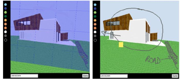
Figure 8. Drawing annotations in space. Drawing a quick straight line on an existing surface generates a temporary grid plane (left) for a user to draw general comments about the whole space. The bright square below the house indicates a text note left to complement the drawing annotations.
