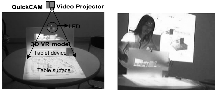
Figure 3 The setup (left) and operation (right) of the spatially-aware navigator
