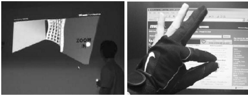
Figure 4 Laser pointer interaction (left) and hand gesture recognition (right)
