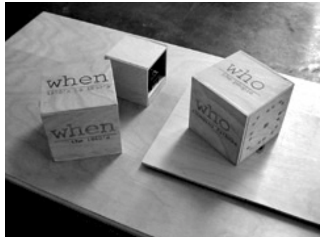
Figure 1. The Navigational Blocks: electromagnets are visible on one face of the “Who” Block positioned on top of the ‘active space’ in front of the (smaller) host Block that is connected to a desktop computer (not shown).
